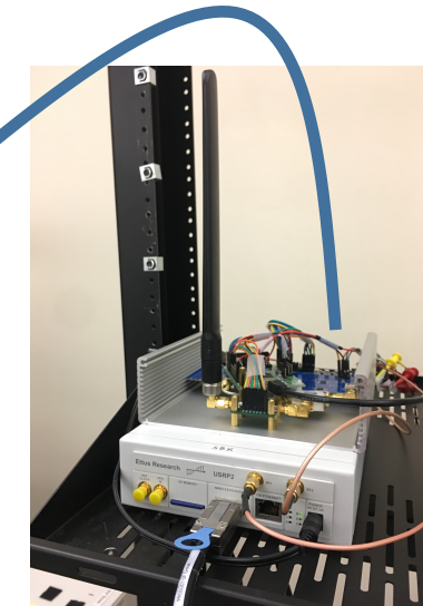
Gen-2 wideband full-duplex radio integrated into COSMOS
